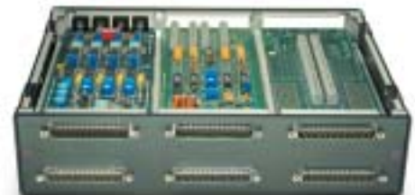
Parallel-port DaqBook/2000X with three expansion slots
